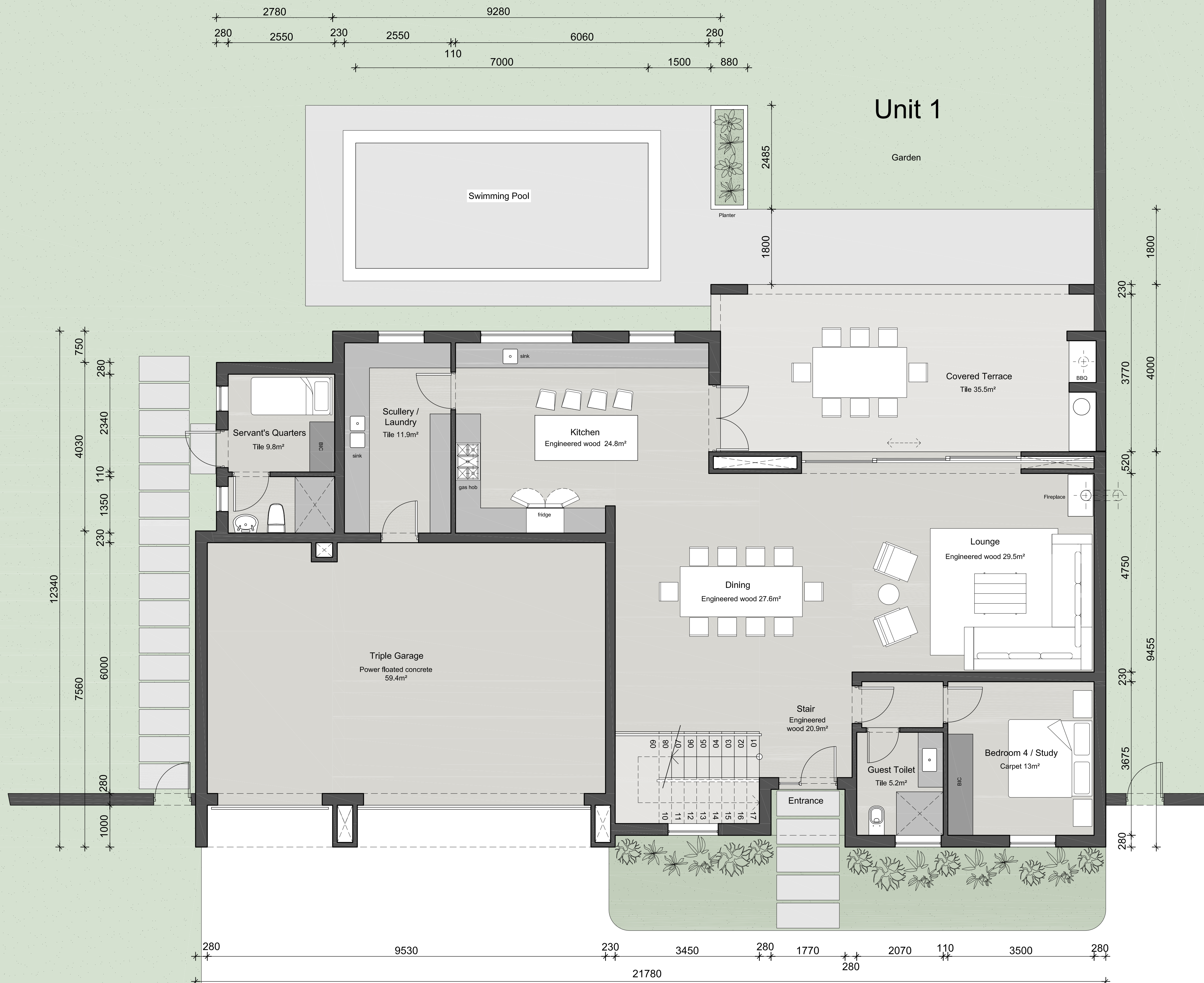
GROUND STOREY PLAN Scale 1:50
